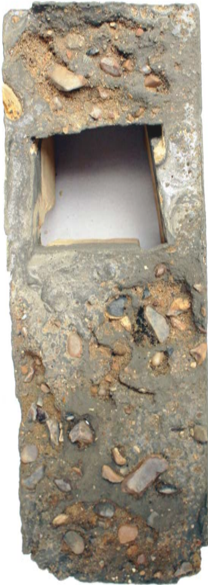
Face [01] rough cast with large aggregate and grey cement
